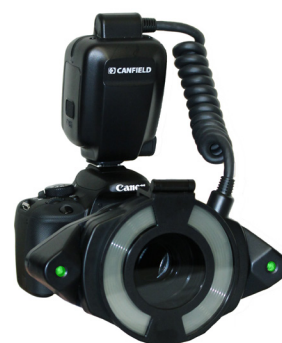
FIGURE 2. (A) A cross-polarizer in the cross-polarized setting covering the lens. One circular polarizer covers the lens opening, while the others, which are polarized at right angles to the lens polarizer, cover the ring flash surrounding the lens opening. (B) The polarizer is removed from the front of the lens enabling plain flash photography without cross-polarization.
