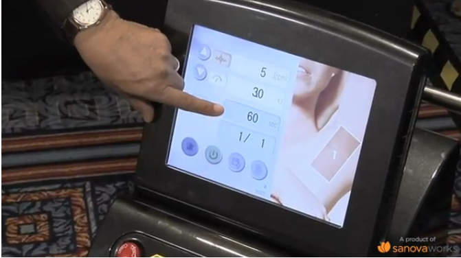
FIGURE 2. The 810 nm diode laser automatically selects the fluence per pulse, total kilojoules, and treatment time.
